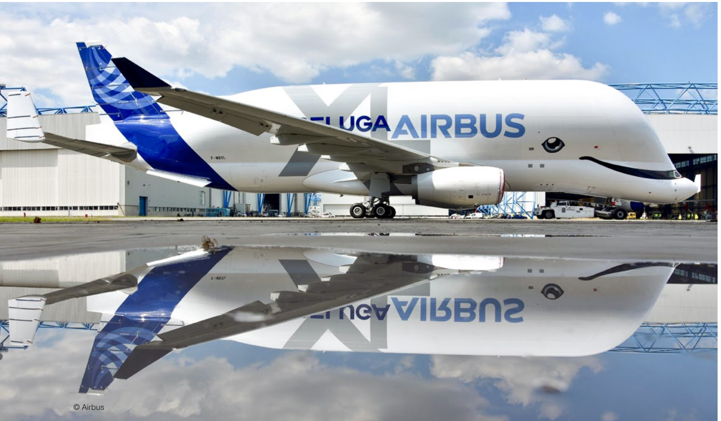
At 63 meters in length, the “smiling” BelugaXL is about seven meters longer than its predecessor, the BelugaST
