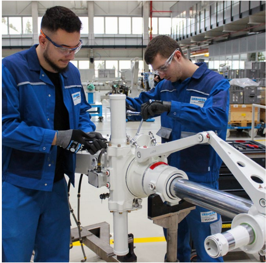
Assembly of an overhauled landing gear at the Liebherr-Aerospace facility in Lindenberg (Germany)
